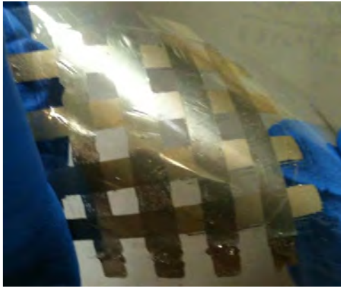
Fig. 1: (a) Schematic of pressure sensor. (b) Photograph of fully printed pressure sensor.
